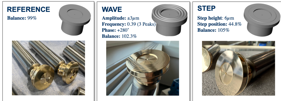
Figure 4.1. Final structured designs with optimized parameters and reference design
