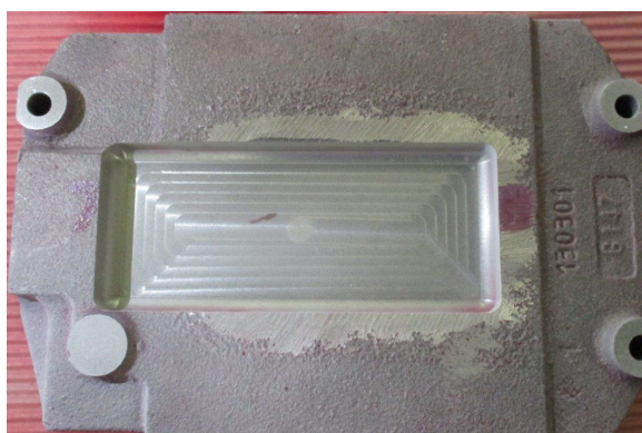
Figure 5.8. Crack on sample 010 with reduced thickness, after 15.888 cycles at 500 bar
