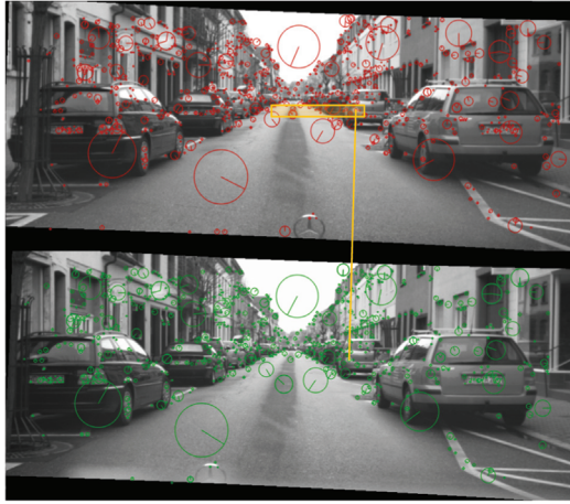
Figure 8.17 Extracted SIFT-features with exemplary geometry-based restriction of matching candidates. By restricting possible matching candidates geometrically, the problem size is significantly reduced.
