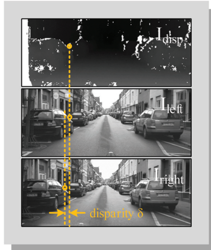
Figure 8.19 Verification of match positions with disparity maps. For rectified images, the horizontal difference of feature positions of a corresponding pixel pair equals the related value of the disparity map. With this technique, it is possible to validate resulting matching lists for datasets with ground truth disparity maps.
