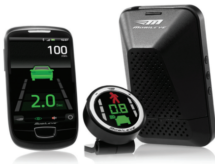
Figure 11.5 Mobileye 560 aftermarket vision-based ADAS.
